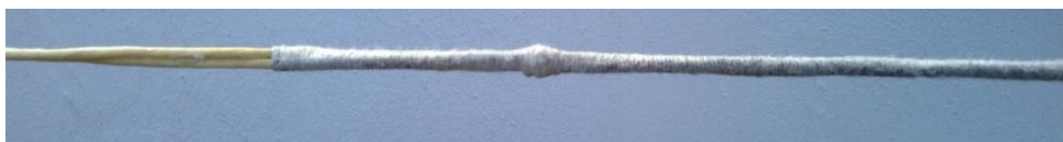
Below: Full-length Hemp fibre string with linen serving (2.5mm diameter at serving)
