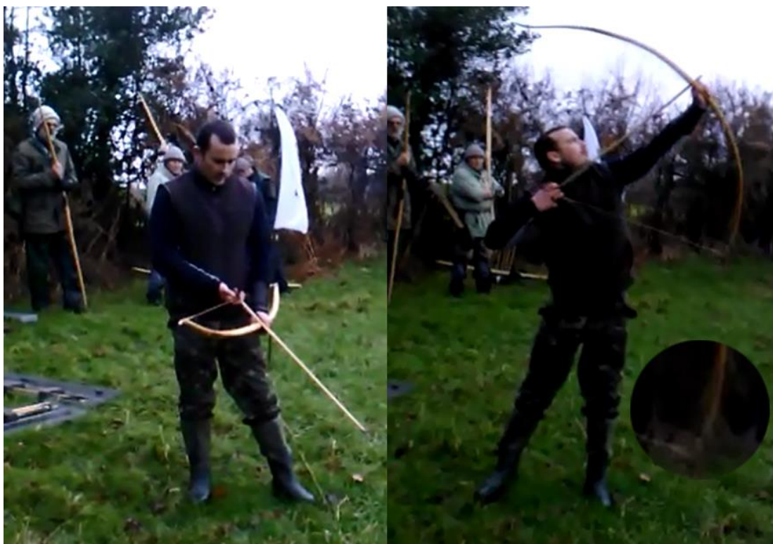
MR X1-3/S2 being drawn to 800mm (31.5 inches). Note the bottom limb failing in tension in the inset and extreme bend induced by the long draw.
