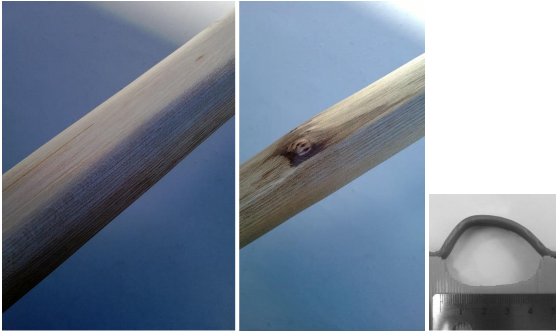
A flat belly, rounded back and a small radiuses edge reflect the profile of original Centre section of MR X1-3
