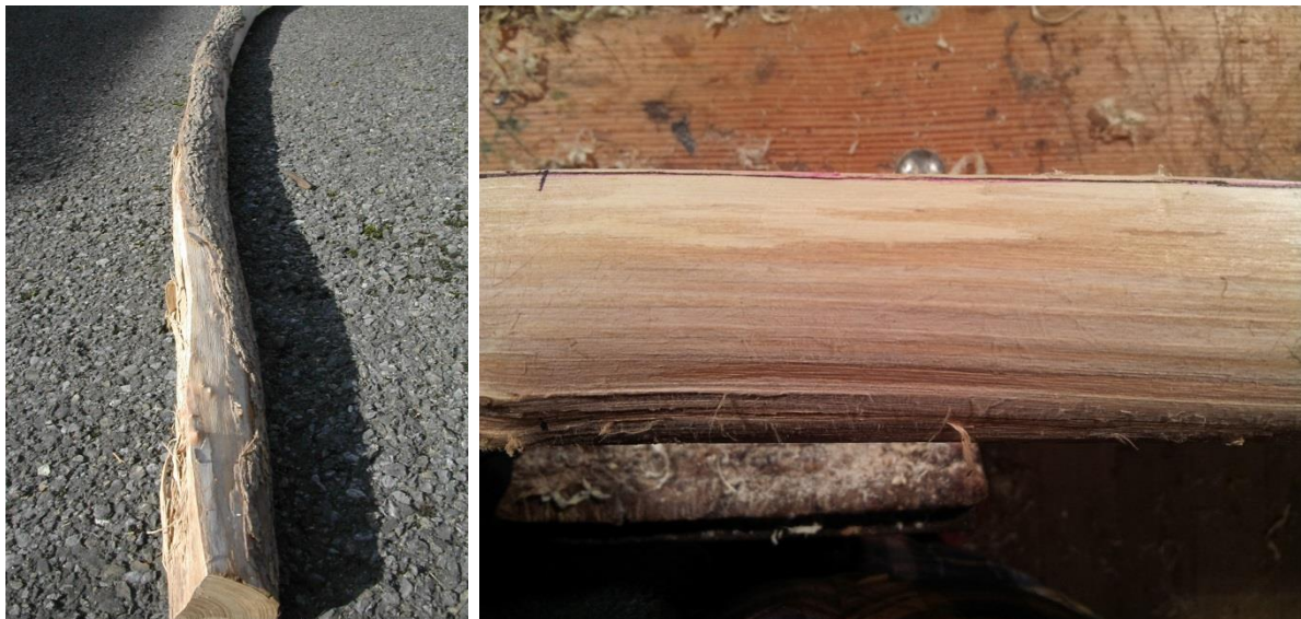
Left: wych elm stave with some of the bark or 'bast' removed. Due to the paucity of clean wych elm staves, some steaming was needed to make them usable. Right: roughed-out stave with the cambium attached.
