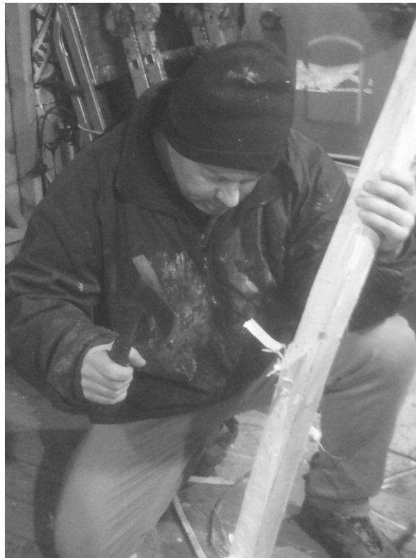
Master bowyer, Jeremy Spencer, roughing out an elm stave for one of the first approximations of bow X1-3
