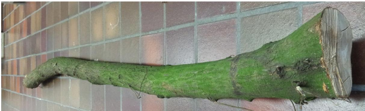
Fig.7. An elm stave that was later corrected using dry heat. Whether it was worth the medieval bowyer’s time to straighten such a character stave is unlikely given the former
