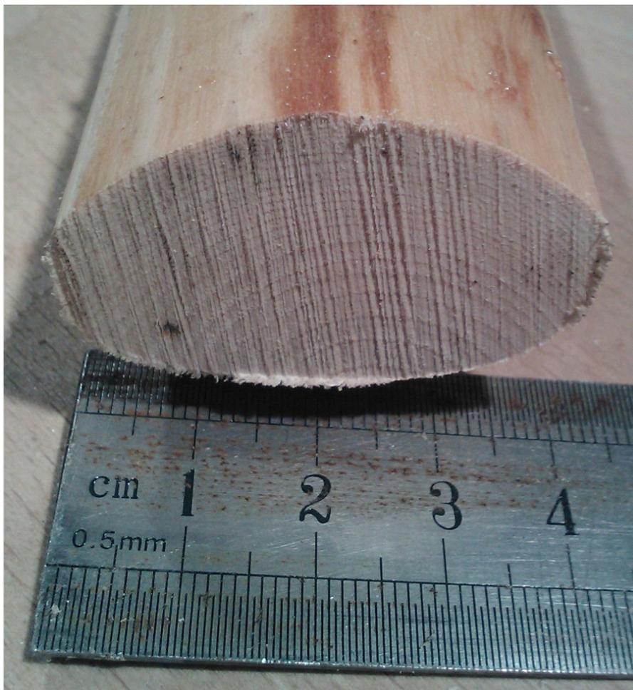
Fig.5. An ideal section for a heavy bow made from a tight ringed shade-grown wych elm stave of 2 ½ in. diameter.
