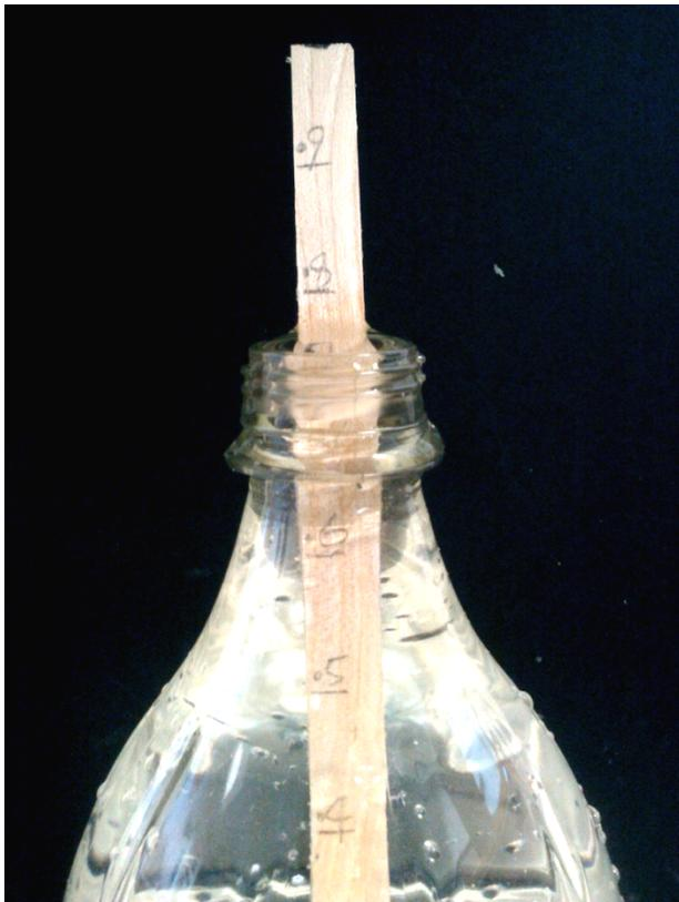
Fig.4. Wych elm density being measured
