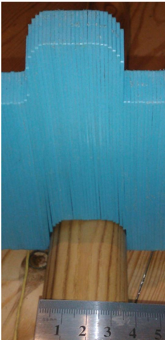
Fig. 6. A flat bellied 115lb ash warbow by talented Czech bowyer, Jaroslav Petrina. The bow is from a large diameter stave so the sides have been heavily rounded to form a pill section, that is with a flat belly and back with hemi-spherical edges. The wood is a dense 0.8 SG.
