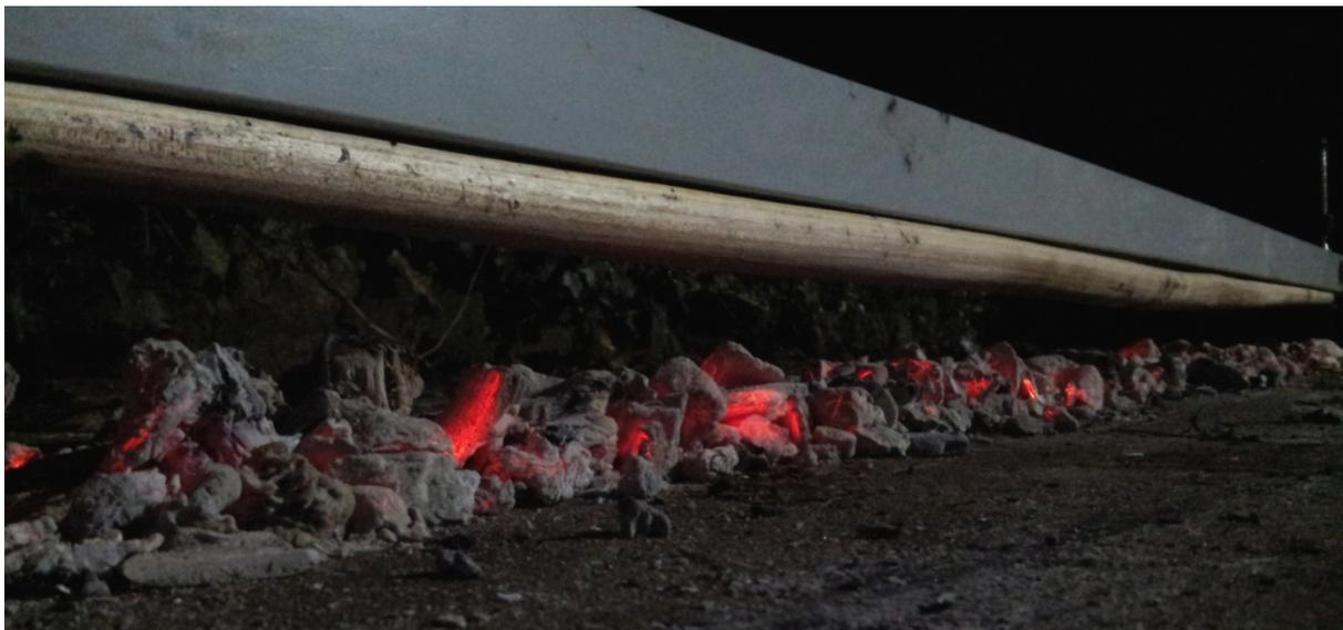
Fig.8. A wych elm stave is simultaneously set straight as its belly is heat-tempered over embers.
